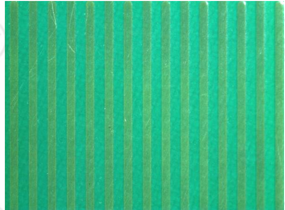
Fig25. Sample PA120510012-2 typical photo 2 after thermal shock test (10 X)
