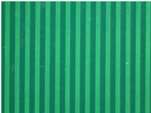
Fig22. Sample PA120510012-2 typical photo1 before thermal shock test (10 X)
